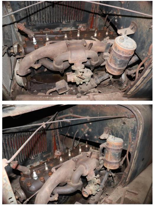
The engine is probably the original flathead six cylinder. The engine size is not known as the model series could not be determined from the VIN. The engine is not operable.
