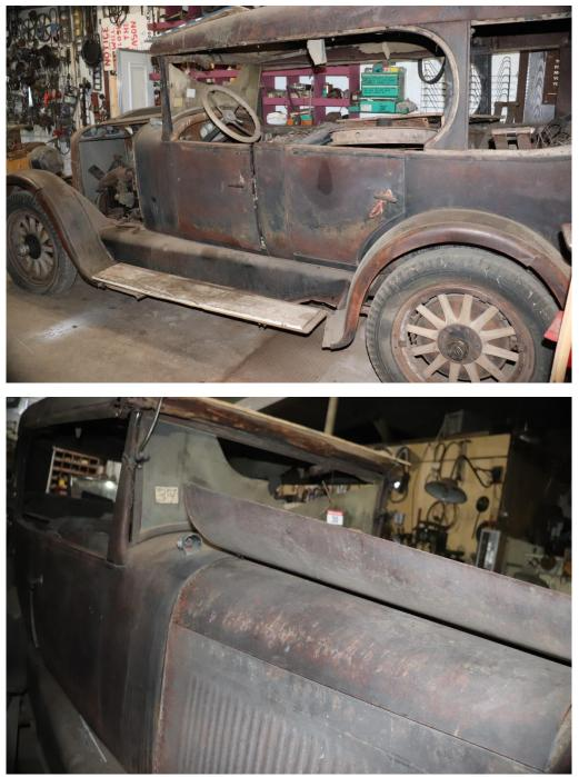
The side panels like the rest of the car are ready for restoration. The glass has been removed or like the windshield, is badly damaged.
